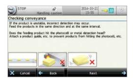
Built-in troubleshooting screens determine the cause of false rejects and provide suggestions to ensure repeatable, stable system performance.
